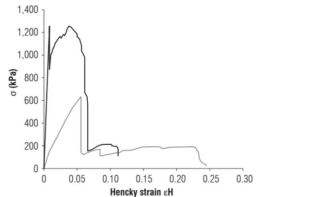
**FIGURE 3.** Typical real stress-Hencky strain curves for puncture test, above: transversely, degrees of maturity 4 and 5; below: longitudinally, degrees of maturity 4 and 5 of sweet passion fruit.
