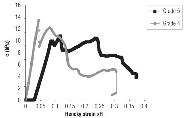
**FIGURE 2.** Typical real stress-Hencky strain curves for unidirectional compression test, longitudinally, degrees of maturity 4 and 5 of sweet passion fruit.
