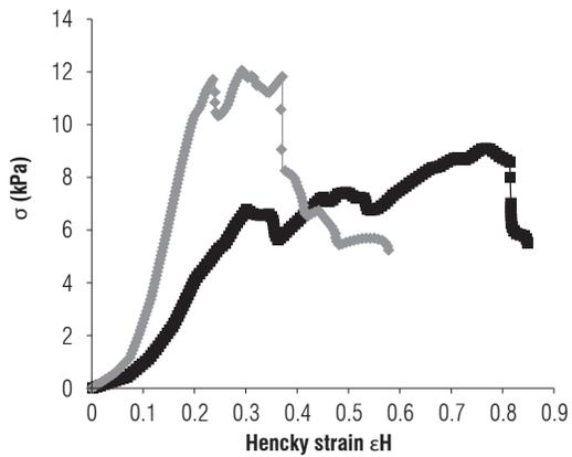
**FIGURE 1.** Typical real stress-Hencky strain curves for a unidirectional compression test, above: in the transversal direction, degrees of maturity 4 and 5 without *mallalon*; below: with *mallalon*, transversal direction, degrees of maturity 4 and 5 of sweet passion fruit.
