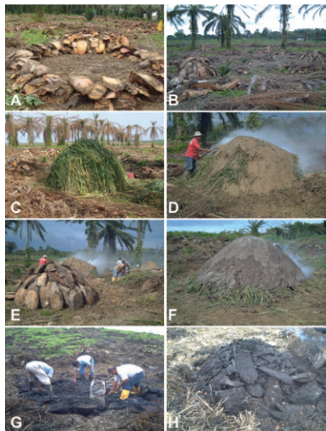
FIGURE 7. Carbonization: palms were felled, chipped and subjected to a carbonization process where piles of biomass consisting mainly of stem chips were burned. These piles of biomass were covered so that the pyrolysis process reduced the airflow to produce charcoal. The fire was then extinguished and the produced charcoal collected. A, stacking of stipes for initial cut; B, formation of stacked pieces of stipes; C, coverage stacked with grass; D, coverage of the pile with soil; E, mount stacked carbonization per plot; F, final Appearance stack operation; G, removal of coal; H, coal obtained at the end of the process.
