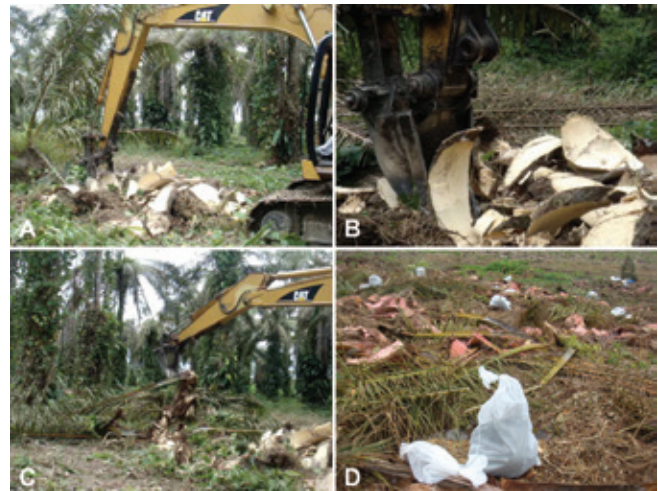
FIGURE 4. Chipping and spreading of palm. A, felled stipes cut by backhoe; B, slice of stipes in the field; C, spreading of the material in the field; D, final appearance of spread-out material.
