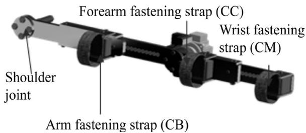
**Figure 3.** Contact areas (securing) of the exoskeleton with the upper limb.
