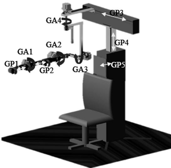
Figure 1. Prototype (degrees of freedom).
