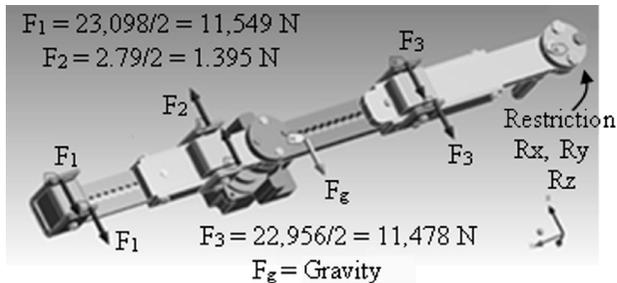
Figure 5. Arm and forearm in loading position and consideration for connection.
