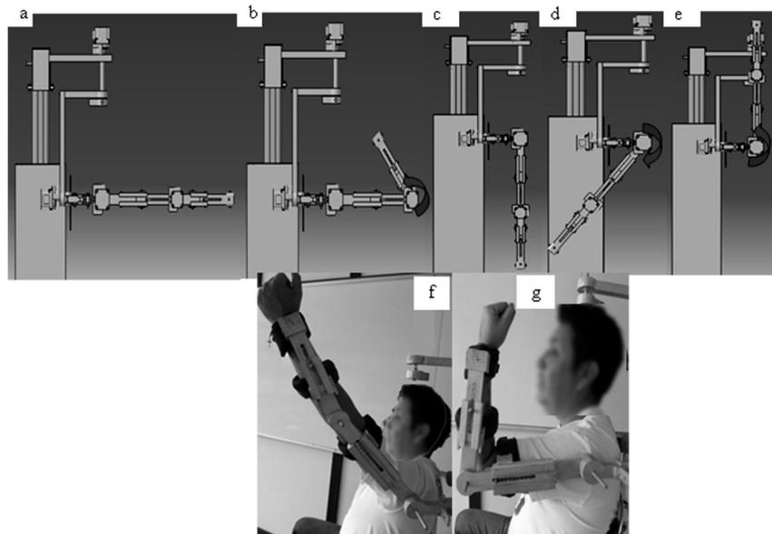
**Figure 26.** Rehabilitation movements: a) Elbow flexion to 0°. b) Maximum elbow flexion. c) Shoulder flexion in the sagittal plane to 0°. d) Maximum shoulder extension. e) Maximum shoulder flexion. f) Patient flexing elbow. g) Patient flexing shoulder.
