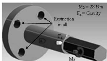
**Figure 10.** Loading position and movement restriction for axis AD2.
