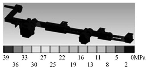
**Figure 16.** First stage of shoulder loading (von Mises stress).
