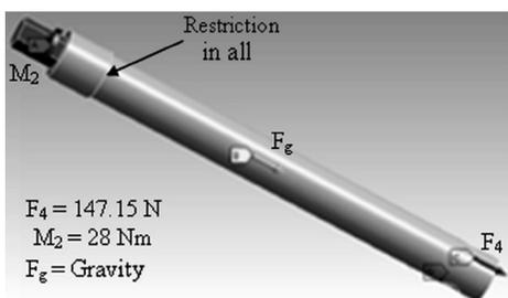
**Figure 11.** Loading position and movement restriction for axis AD4.
