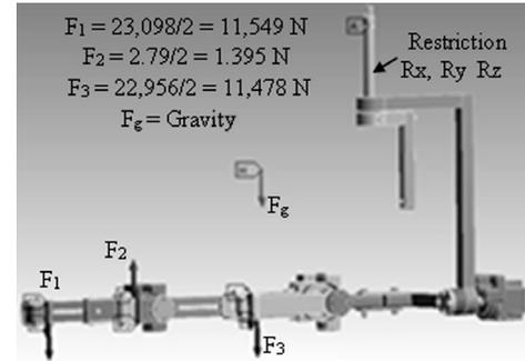
Figure 7. Shoulder in second loading position.
