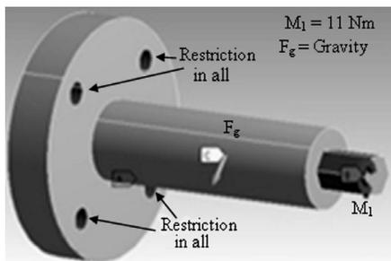
**Figure 9.** Loading position and movement restriction for AD1 axis.
