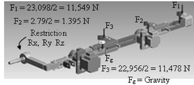
Figure 6. Shoulder in first loading position.
