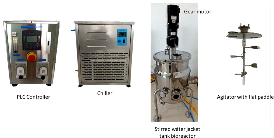
Figure 1. Design coffee stirred tank bioreactor equipment.
