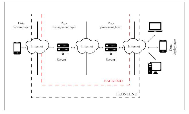
**Figure 8.** System architecture. Source: Elaborated by the authors
