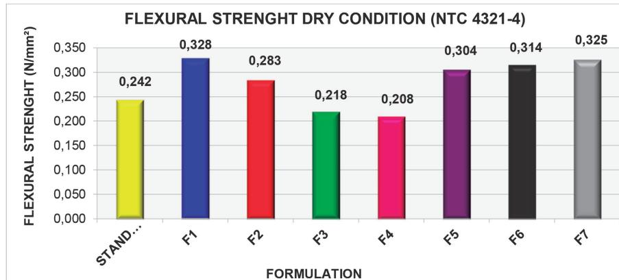
Figure 9. Flexural strength in dry condition formulations.
