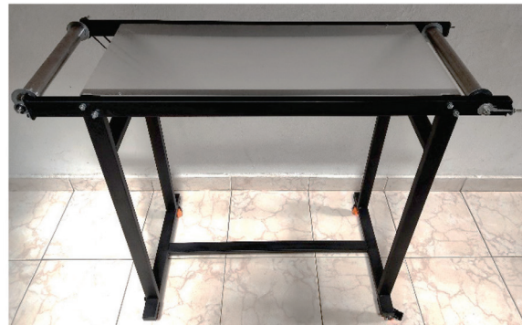
Figure 14. Structure built for conveyor belt
