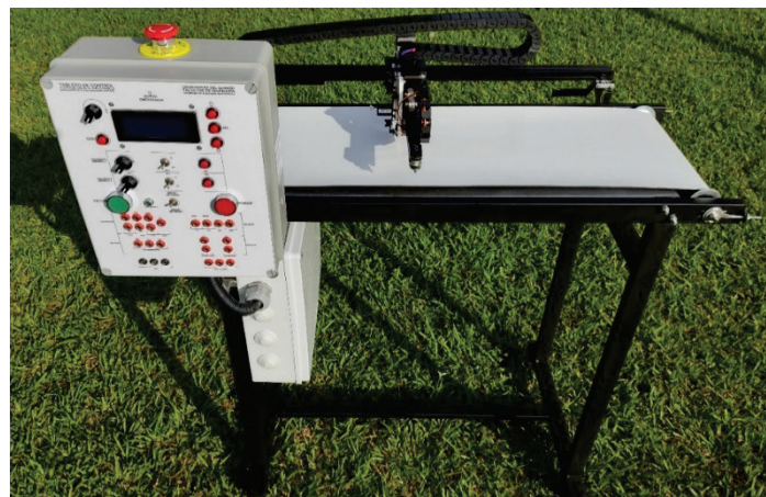
Figure 35. Flying-cutting plant implemented
