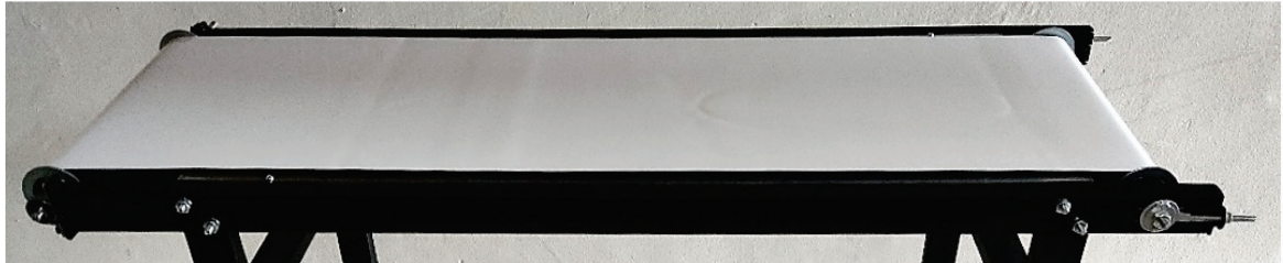
Figure 15. Conveyor belt placed on the rollers of the conveyor belt structure
