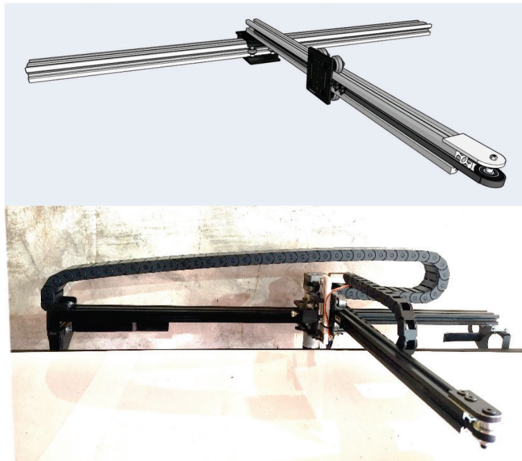
Figure 16. SketchUp 3D model and real implementation for cutting system
