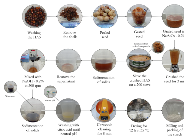
Figure 1: Process of wet alkaline starch extraction.
