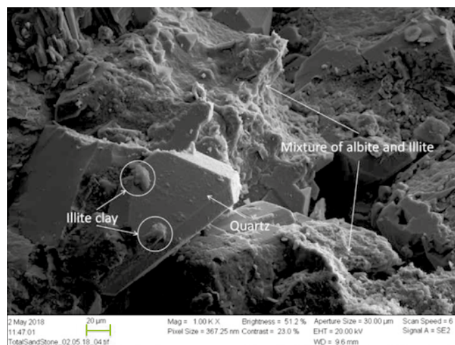
Figure 13. SEM photo taken from the sandstone material used. Silicates such as clay, quartz, and feldspars were identified magnification 1000X.
