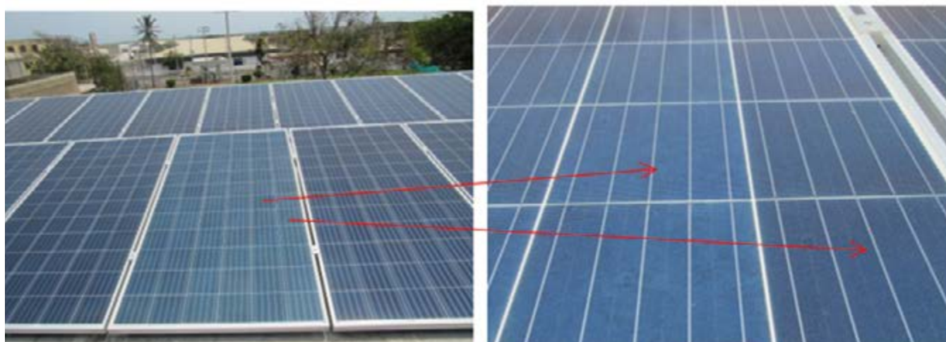
Figure 5. Discoloration between cells in the same PV module
