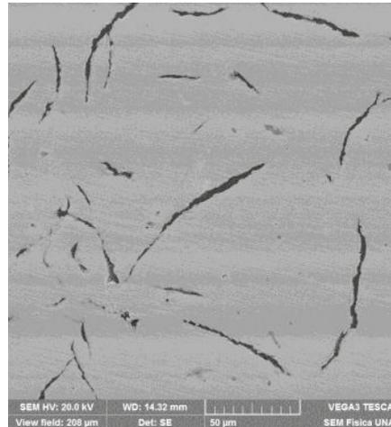
**Figure 1.** Micrograph of gray cast iron without biodiesel exposure. 2000X. Polished with alumina 10 μm. Lamellar graphite with pearlitic phase in the matrix.
