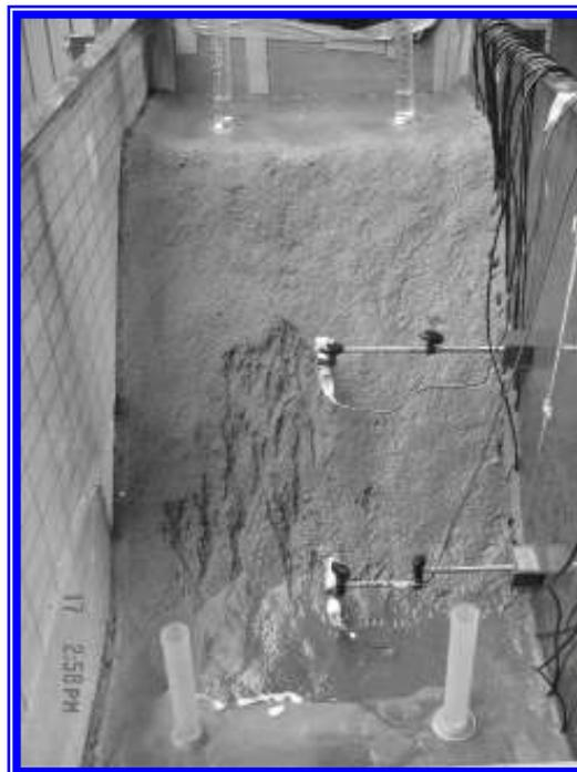
**Figure 7.** Transducer configuration to measure displacement. Model Test No. 07
