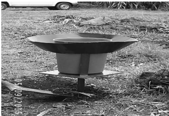
Figura 6. Colectores de polvo Figure 6. Dust collectors
