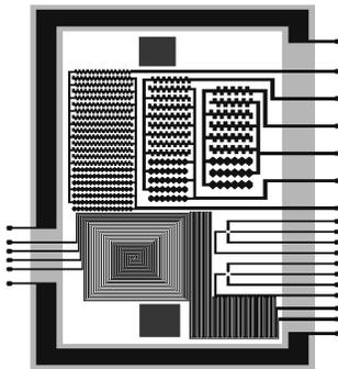
**Figure 2.** Mask diagram including the three required layers to process the microchip. The two red-square regions have a side length of 900 (top) and 1000 (bottom)  $\mu\text{m}$  and serve to build the inlet and outlet holes by micromachining. The green rectangle of 800  $\mu\text{m}$  in width will be used to pattern the photoresin. The blue level contains diverse electrode microarrays and will outline the metal layer
