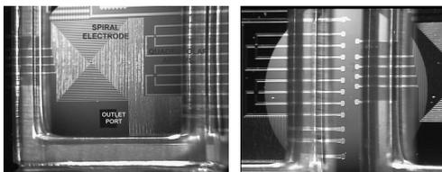
**Figure 13.** Photographs of the spiral and quadrupolar microelectrode arrays (left) and a detail of their pads (right) before dicing. Photoresin transparent walls can be clearly observed, as well as electrode wires crossing under them to connect the electrodes themselves to the external pads
