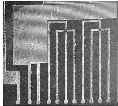
**Figure 9.** View of the platinum meandering wire. The assessed resistor value was 6895  $\Omega$  while its measured value was 6800  $\Omega$  at 25  $^{\circ}\text{C}$
