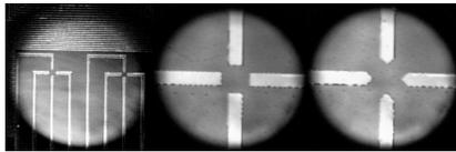
**Figure 8.** Quadrupoles of 50  $\mu\text{m}$  in electrode width and 100  $\mu\text{m}$  in separation. On the left a total view of both microstructures is shown, while the other two photographs reproduce a detailed view of the square and triangular microelectrodes
