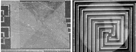
**Figure 7.** Total view of the square spiral microarray with a side length of 2700  $\mu\text{m}$  (left), and partial view of the central part of the same platinum spiral (right)
