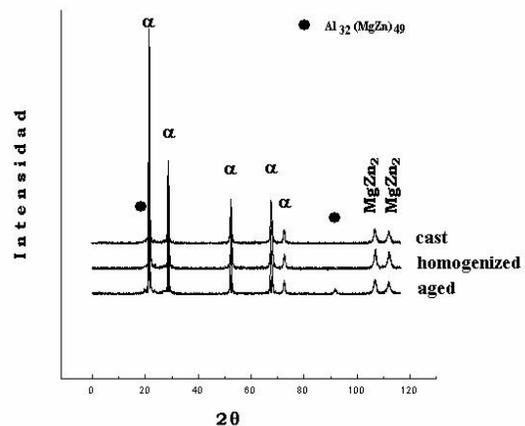
**Figure 3.** Phases identified by X-ray diffractometry in the AlMgSiZn ingots
