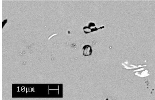
**Figure 4.** Precipitates observed in AlMgSiZn alloy aged
