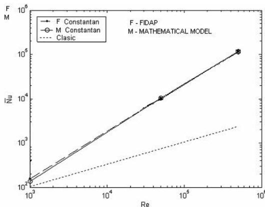
**Figure 12.** Comparison between the classic average Nusselt number and average Nusselt number obtained from FIDAP solution and the semi analytical model (Oil MIL 7808 - Constantan,  $Re = 1 \times 10^3$ ,  $L^* = 0.5$ )
