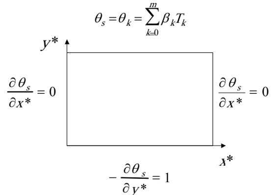
**Figure 2.** Two dimensional heat conduction problem at the plate
