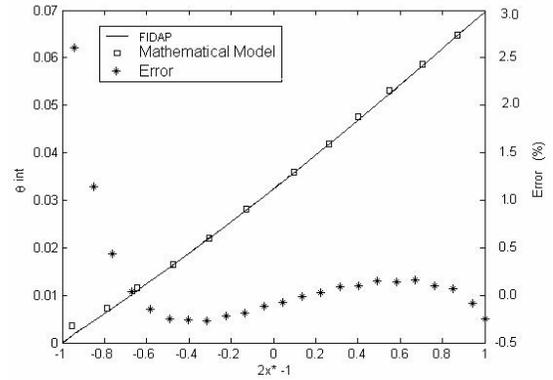
**Figure 8.** Temperature at the interface and error from the mathematical model and FIDAP solution
