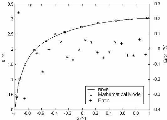
**Figure 11.** Temperature at the interface and error from the mathematical model and FIDAP solution. (Oil MIL 7808 - Constantan,  $Re = 1 \times 10^3$ ,  $L^* = 0.5$ )
