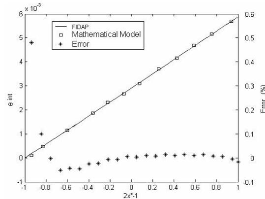
**Figure 5.** Temperature at the interface and error from the mathematical model and FIDAP solution (Oil MIL 7808 - Constantan, Re = 5x10<sup>5</sup>, L\*=0.5)
