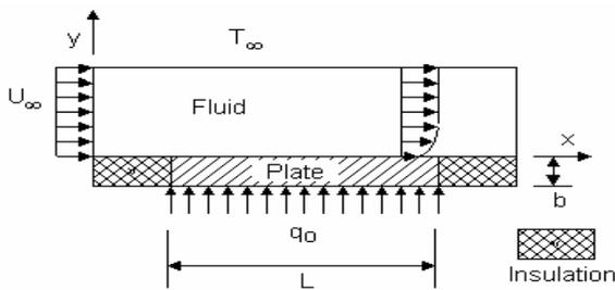
Figure 1. Schematic of a rectangular plate under the influence of a laminar flow
