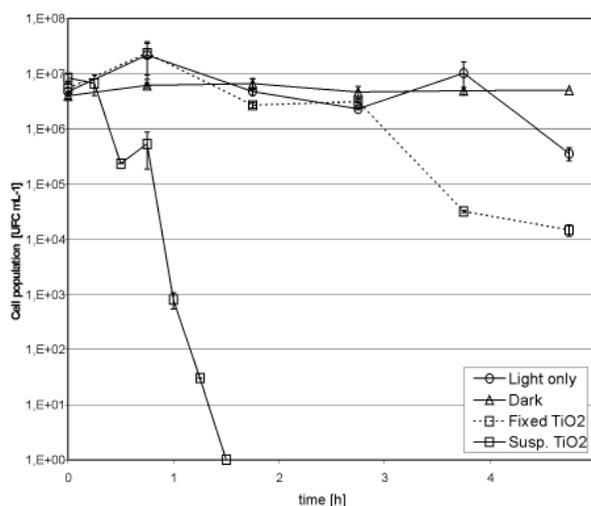
**Figure 2.** UFC mL<sup>-1</sup> comparison between suspended and fixed TiO<sub>2</sub>: Triangles represent the control experiment, without light and without TiO<sub>2</sub>. Circles represent the experiment with irradiation only, while squares with a dashed and full line represent experiments with fixed and suspended TiO<sub>2</sub>, respectively
