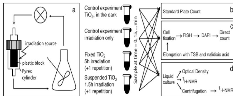
**Figure 1(a).** The Photocatalytic reactor. The total illuminated volume was 43 mL, the temperature was maintained at 32°C and a peristaltic pump ensured a flow of 150 mL  $min^{-1}$ . Irradiation was at about 40  $W/m^2$  of UV-light at 254 nm. (b-d) Flow diagram of the experiments
