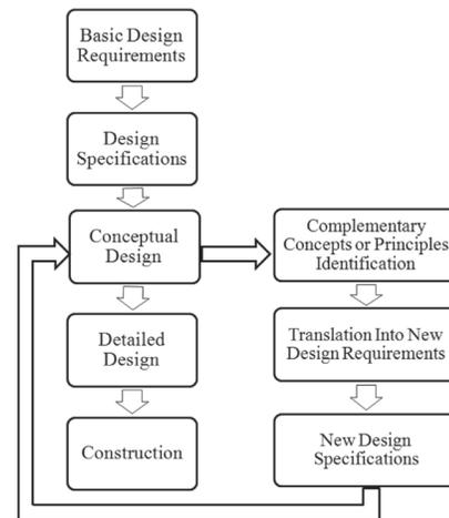
**Figure 2.** Modified design cycle
