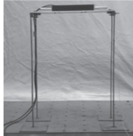
**Figure 1.** Structure with active mass damper control system (AMD)
