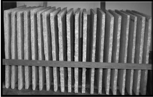
**Figure 4.** Specimen conditioning
