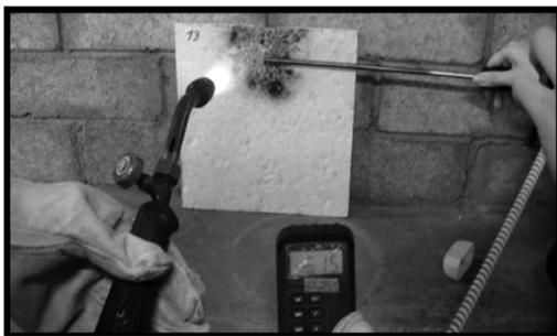
**Figure 7.** Recipanel fire test
