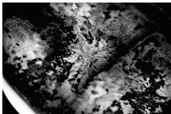
Figure 5. Microphotography with a zoom of 40X, sample of conventional rice. Zone with darkness gray corresponds to polysaccharides distribution.
