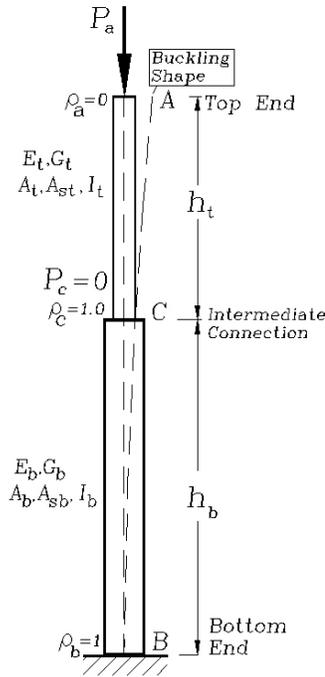
**Figure 7.** Example 4: Single-stepped cantilever column (Timoshenko & Gere [2], p. 115).
