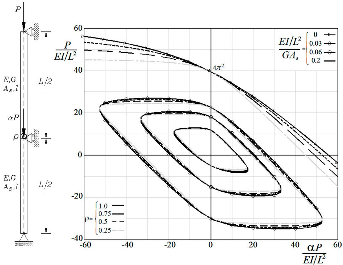
**Figure 2.** Shear effects (Haringx approach) and semirigid connection at mid-support ( $r_c$ ) on the buckling loads ( $P$  and  $aP$ ) of the single-stepped column ABC of Problem 1 [assuming that:  $r_a = r_b = 0$ ,  $E_t I_t = E_b I_b = EI$ ,  $GA_{st} = G_b A_{sb} = GA_s$ , and  $h_t = h_b = L/2$  in the model shown in Fig. 1(a)].
