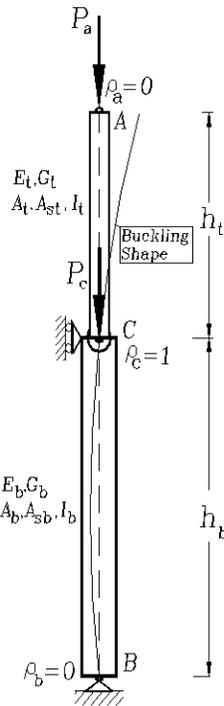
Figure 6. Example 3: Single-stepped column simple supported at C and B and top sidesway
