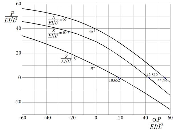
Figure 4. Interaction diagrams  $P/(EI/L^2)$ -vs- $\alpha P/(EI/L^2)$  for the column of Example 2 [for the particular case of  $h_t = h_b = L/2$ ,  $k_c = 0$ ,  $G_t A_{st} = G_b A_{sb} = \infty$  and  $E_t I_t = E_b I_b = EI$ ] assuming that  $P_a = P$  and  $P_c = \alpha P$  with an intermediate elastic support with  $S_c/(EI/L^3) = \infty, 100$ , and  $0$
