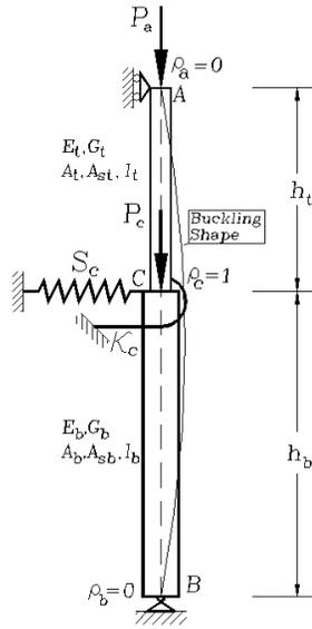
Figure 3. Example2: Single-stepped column simply supported at A and B
