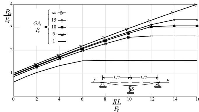
Figure 5. Variations of the critical load of a simply supported column with the stiffness of the intermediate elastic support  $S$  and its shear stiffness  $GA_s$  ( $P_e = p^2 EI/L^2$ ) using the Haringx approach
