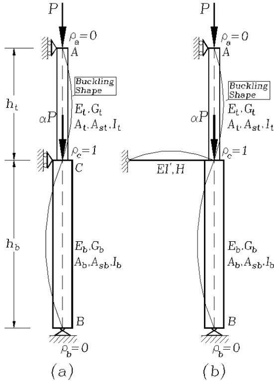
**Figure 1.** Example 1. Single-stepped column (according to Timoshenko & Gere [2], pp. 66-70): (a) on three supports with hinged ends; and (b) on end supports and rigidly connected at C to transverse beam with its far end hinged.
