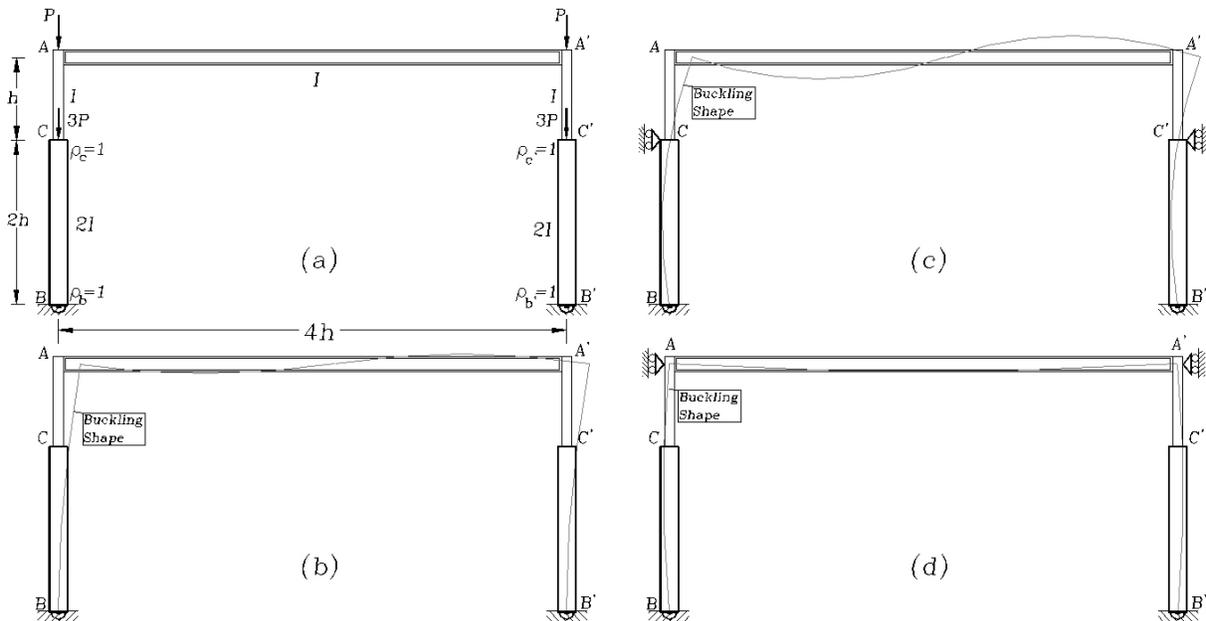
**Figure 8.** Example 5: Minimum lateral bracings for a simple bent frame with stepped columns: (a) structural model; (b) buckling mode with sidesway between A and B uninhibited; (c) buckling mode with sidesway between C and B totally inhibited; and (d) buckling mode with sidesway between A and B totally inhibited
