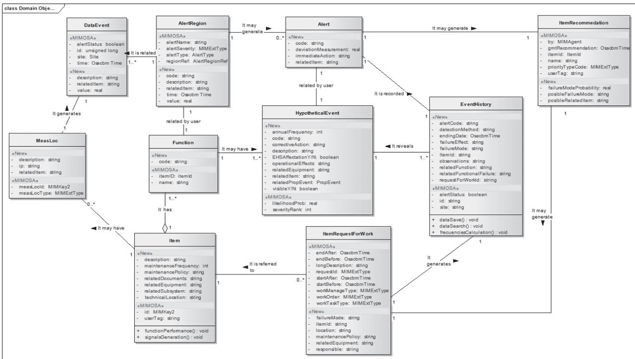
Figure 2. UML Data model of the integrated system
