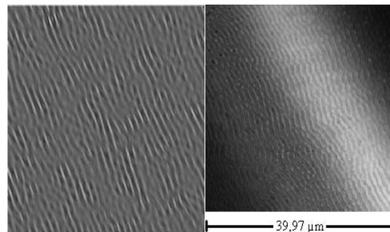
Figure 4. Comparison between simulation for a  $186 \times 186$  lattice size using a Lattice-Boltzmann simulation, left panel, and experimental result, right panel. Simulation result elaborated in gnuplot [32], and right figure obtained using a confocal laser microscope.
