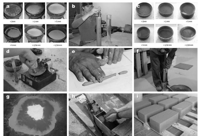
Figure 6. Stages of characterization of raw materials and preparation of CEBs. (a)-(b) Combined sieve and hydrometer analyses of the clay-rich material. (c) Sieve analyses of the gypsum mining waste. (d)-(e) Test of the Atterberg's limits (limits of consistency). (f) Proctor Compaction test. (g) Mix of materials. (h) Mix in the *Cinva-Ram* block-making machine before pressing process. (i) Resultant set of CEBs
