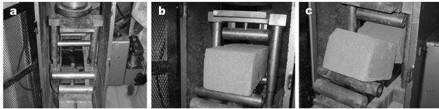
Figure 9. Flexural strength test set up, showing experimental set up and resultant CEBs after testing
