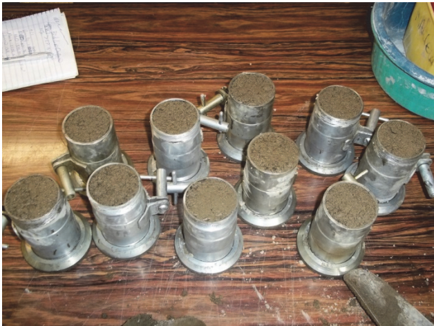
Figure 4. Cylindrical specimens of dimension 5 cm x 10 cm.
