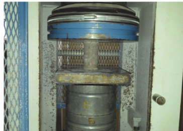
Figure 6. Equipment used for assessing the physical properties of the specimens: (a) drying of the specimen in the greenhouse, (b) determining the mass of the specimen using a hydrostatic weighing-machine and (c) compression test in the ELE machine.
