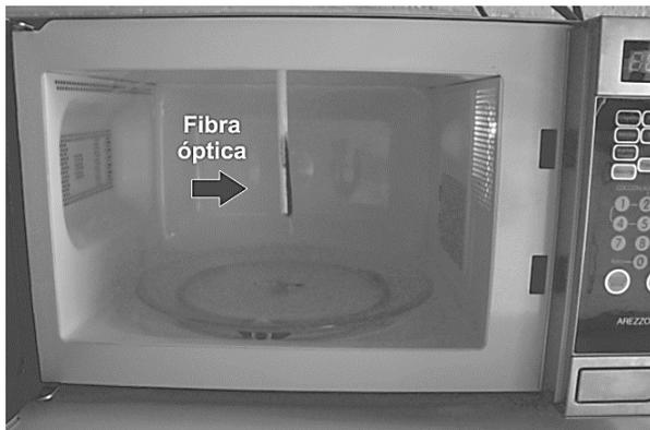
Figure 2. Location of the FBG sensor inside the home microwave oven.
