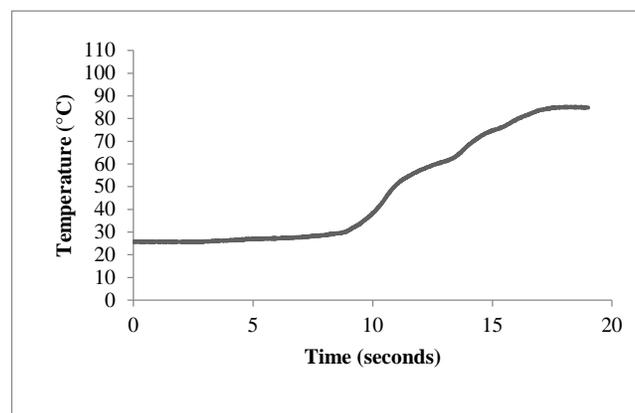
Figure 4. Heating curve of the liquid coffee extract obtained by optical fiber sensor.
