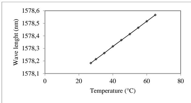
Figure 1. Calibration of the FBG sensor using a calorimeter.
