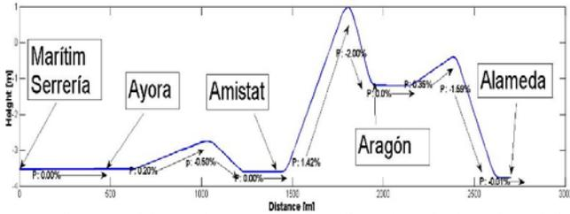
Figure 2. Vertical layout between Marítim Serreria and Alameda and the stations (stops) in between them.
