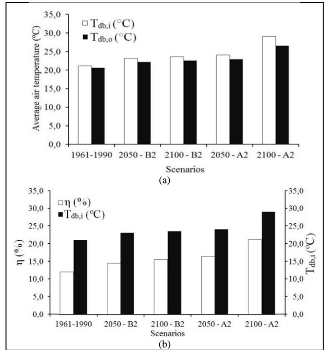
Figure 7. Behavior of average air temperature before ( $T_{db,i}$ ) and after ( $T_{db,o}$ ) crossing the wetted porous plate (a) and evaporative cooling efficiency ( $\eta$ ) due to the variation of the air temperature ( $T_{db,i}$ ) before crossing the wetted porous plate (b) according to the estimated average air temperature for the period of 1961-1990 and according to the B2 and A2 scenarios (IPCC, 2013), for the years 2050 and 2100. Source: The authors.
