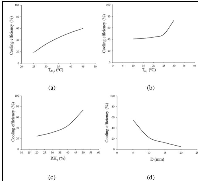
Figure 6. Sensitivity of cooling efficiency ( $\eta$ , °C) to inlet dry bulb temperature ( $T_{db,i}$ , °C, A), inlet water temperature ( $T_{w,i}$ , °C, B), inlet air relative humidity ( $RH_i$ , %, C) and expanded clay average diameter ( $D$ , mm). Source: The authors.
