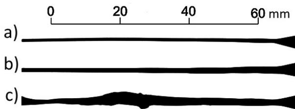
Figure 17. Shape of focusing tube wear with corundum after: a) 5 min, b) 10 min. c) 20 min.
