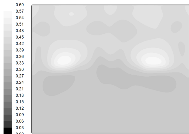
Figure 10. Velocity profile on the grate (m/s) after optimization. Source: The authors.
