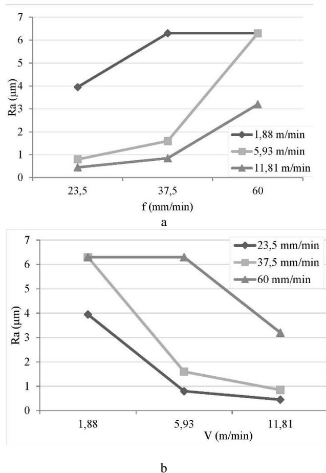
Figure 2. Effect of feed rate (a) and cutting speed (b) on the surface roughness of the workpiece.
