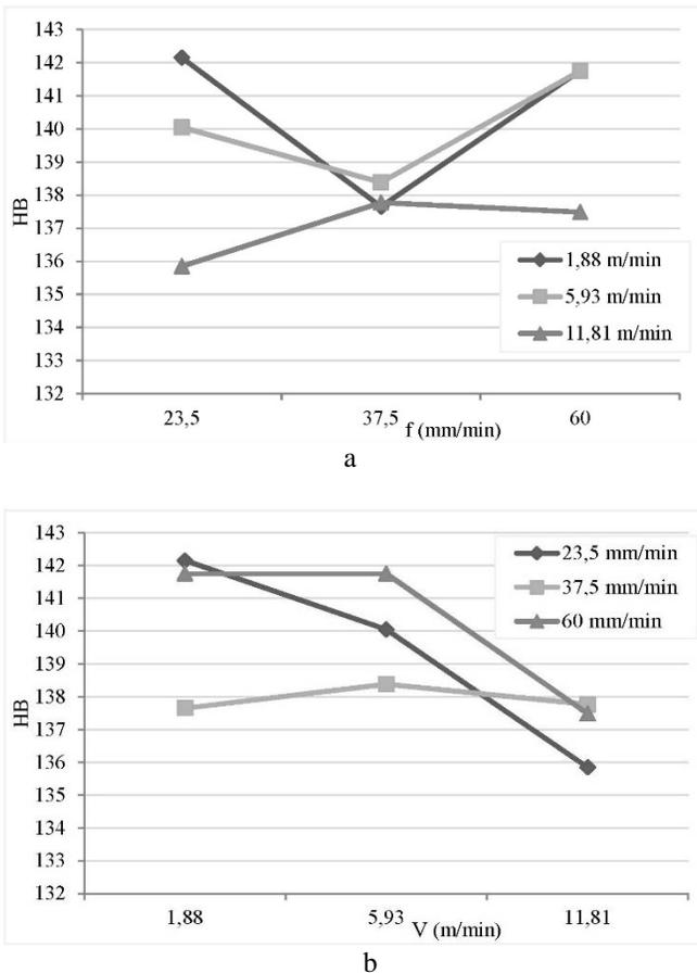
Figure 1. Effect of feed rate (a) and cutting speed (b) on the hardness of the workpiece.
