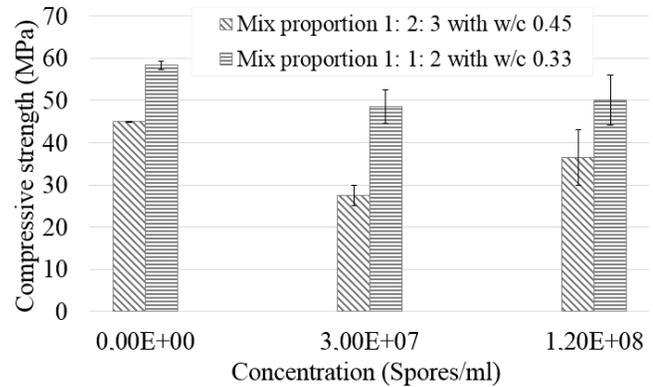
Figure 7. Compressive strength of concretes. Source: The authors.
