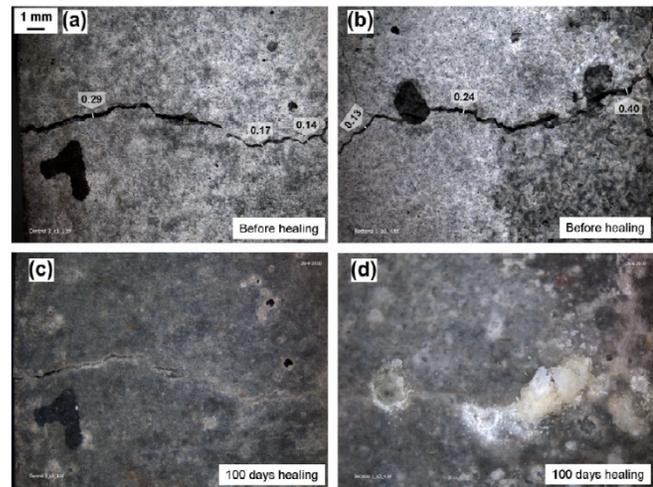
Figure 6. Stereoscopic images of crack-healing process in control mortar specimen before (a) and after 100 days healing (c), in bio-chemical agent-based specimen before (b) and after 100 days healing (d). Source: [3].
