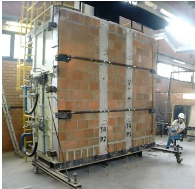
Figure 2. Experimental setup: columns embedded in masonry wall Source: Authors
