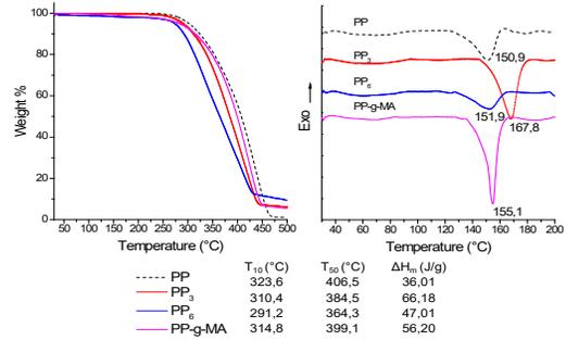
Figure 5. a) Results of TGA and b) DSC obtained from the starting materials.
