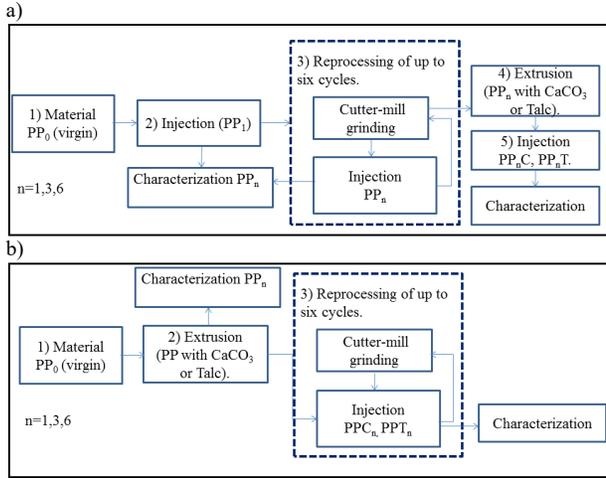
Figure 1. a) Stages for process of obtaining compounds PP<sub>n</sub>M. b) Steps for process of obtaining compounds PPM<sub>n</sub>. Source: The authors.
