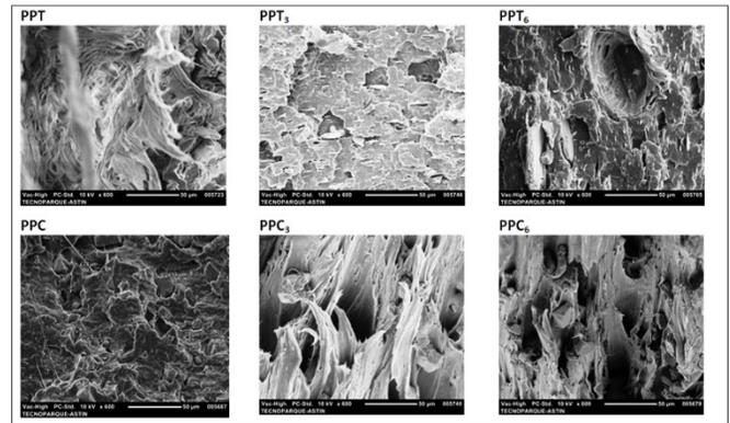
Figure 6. SEM micrographs taken from fracture surfaces of PPM<sub>n</sub> composites at a magnification of 600x.
