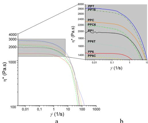
Figure 4. a) Dependence of the apparent viscosity on the shear rate per cut at 190 °C, of composites of the first and the sixth injection cycle. b) A magnification of the region of shear rate from 0 to 10 s<sup>-1</sup>.
