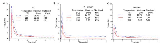
Figure 2. Rheogram for the PP and composites a) PP, b) PPC y c) PPT. Source: The authors.
