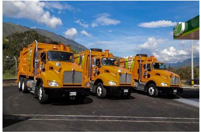
Figure 1. Vehicles run on Natural Gas solid waste collection trucks of EMVARIAS of Medellín.
