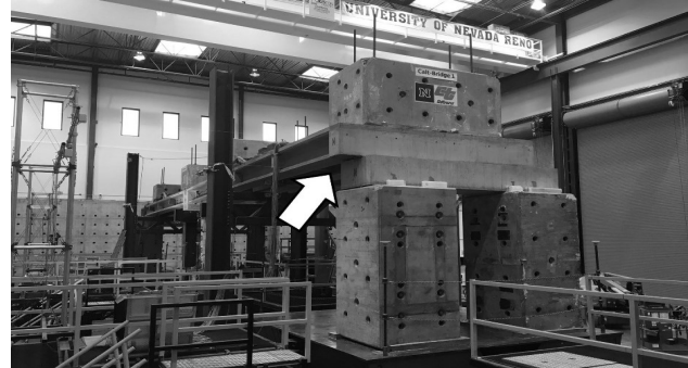
Figure 12. Deformed configuration of bridge model at end of tests. Source: The Authors.
