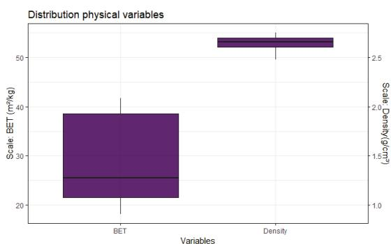
Figure 6. Density and Specific surface area (BET) for calcined clays with high silicon oxide content.
