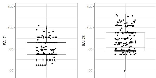
Figure 7. SAI values for calcined clays with high silicon oxide content at 7 and 28 days.
