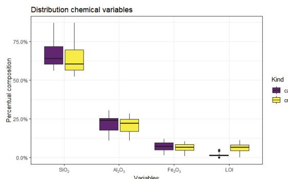
Figure 4. Chemical composition in oxides for raw (cr-yellow) and calcined (cal-purple) state clays with high silicon oxide content.
