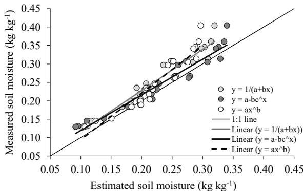
Figure 5. Relationship between soil moisture ( $\theta_m - \text{kg kg}^{-1}$ ) measured by gravimetric method and determined with the capacitive sensor. Source: The authors.
