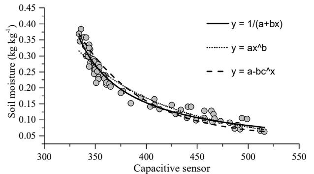
Figure 4. Relationship between gravimetric soil moisture ( $\theta_m - \text{kg kg}^{-1}$ ) and the output signal of the capacitive sensor v1.2. Source: The authors.
