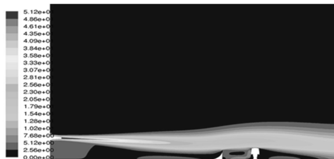
Figure 14. Results for the critical case study: speed magnitude contours for the aircraft engine (m/s), deflector and Aerotren. Source: Authors.
