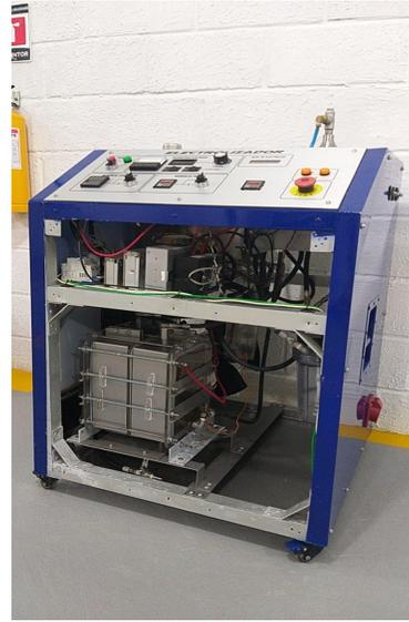
Figure 3. Hydrogen generation bench.
