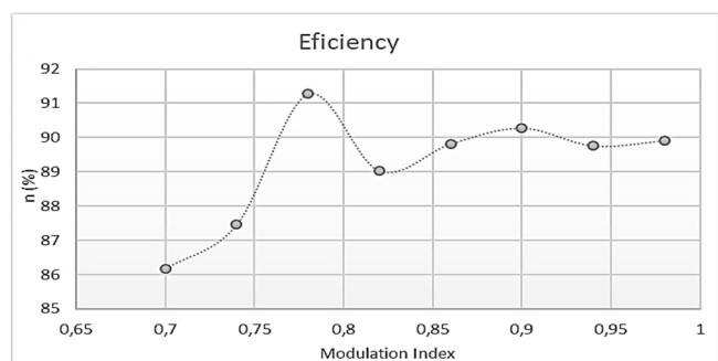
Figure 16. Modulation index versus efficiency in open loop. Source: The Authors.
