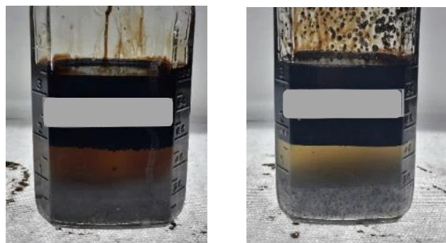
Figure 5. Surfactant & Mutual solvent effects in detergency tests for F1. Source: The authors.
