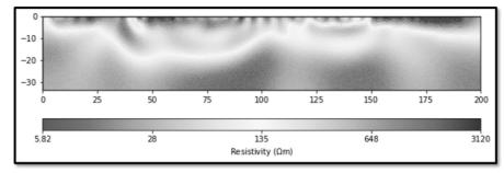
Figure 9. ERT from the geoelectric data and the inversion process described in this paper. Source: pyGIMLi.
