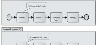
Fig. 2. Pointcut represented with annotation elements and indicating the join points.
