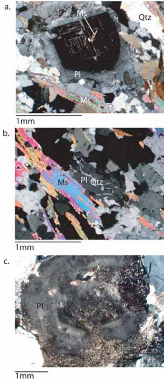
**Figure 7.** Photomicrographs illustrating relict igneous textures in leucosomes lithologies, Nason Ridge Migmatitic Gneiss, WA. a. Subidioblastic simple zoning in plagioclase. b. Quartz-plagioclase myrmekitic intergrowth. c. Idioblastic oscillatory zoning in plagioclase.
