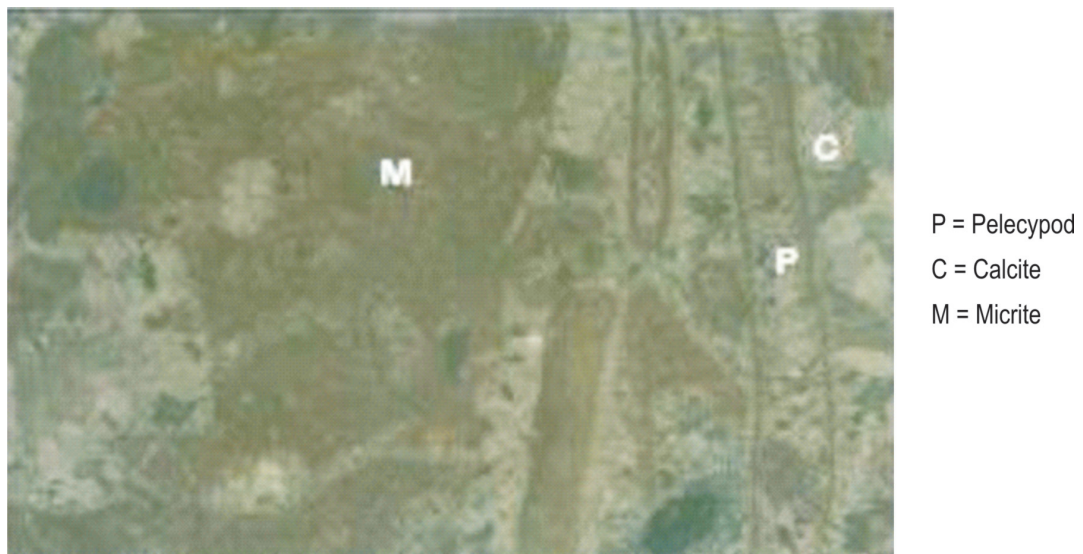
Plate 4: Photomicrograph of Ibese limestone (Depth 37.5m)
