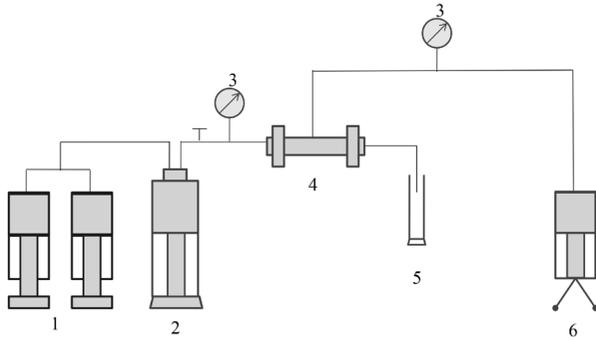
\*Note: 1-Pump. 2-Intermediate container. 3-Pressure gage. 4-Core holder. 5-Measuring cylinder. 6-Confining pressure pump.
