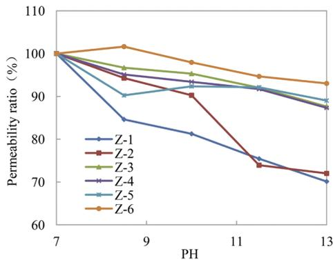
Figure 9. Alkaline sensitivity experiment results.
