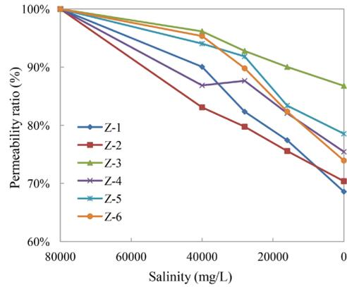
Figure 8. Salt sensitivity experiment results.
