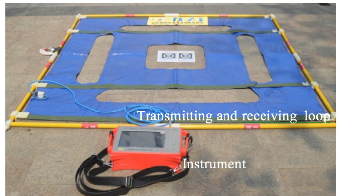
Figure 5. YCS360 electromagnetic system.
