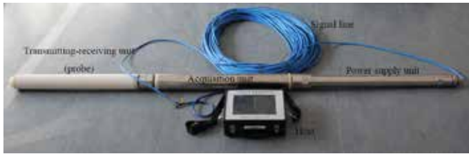
Figure 4. Borehole TEM instrument.
